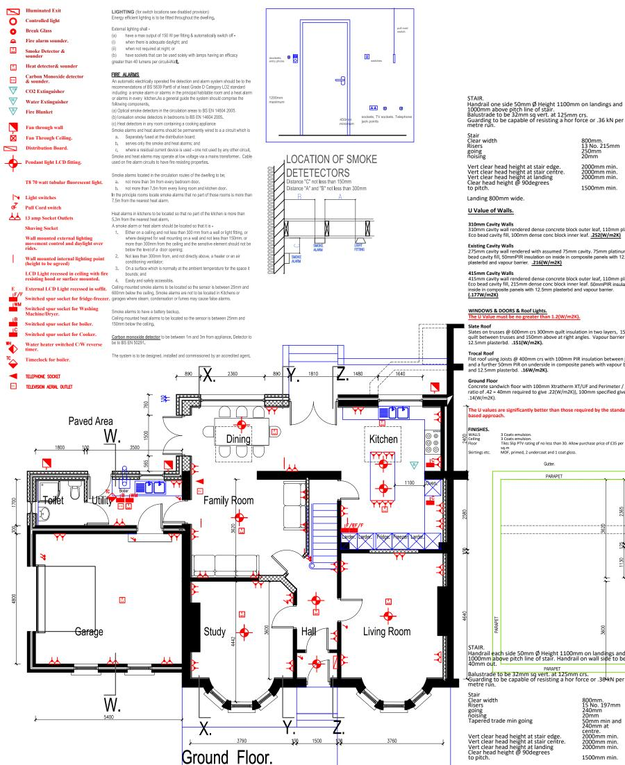
800mm. 13 No. 215mm 250mm 20mm 2000mm min. 2000mm min. 2000mm min. 1500mm min. 310mm cavity wails rendered dense concrete block outer leaf, 110mm plat Eco bead cavity fill, 100mm dense conc block inner leaf. <u>.252(W/m2K)</u>
